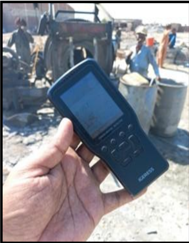
Monitoring of Air Pollution level during execution of work at Zone A Yard with the help of Formaldehyde
