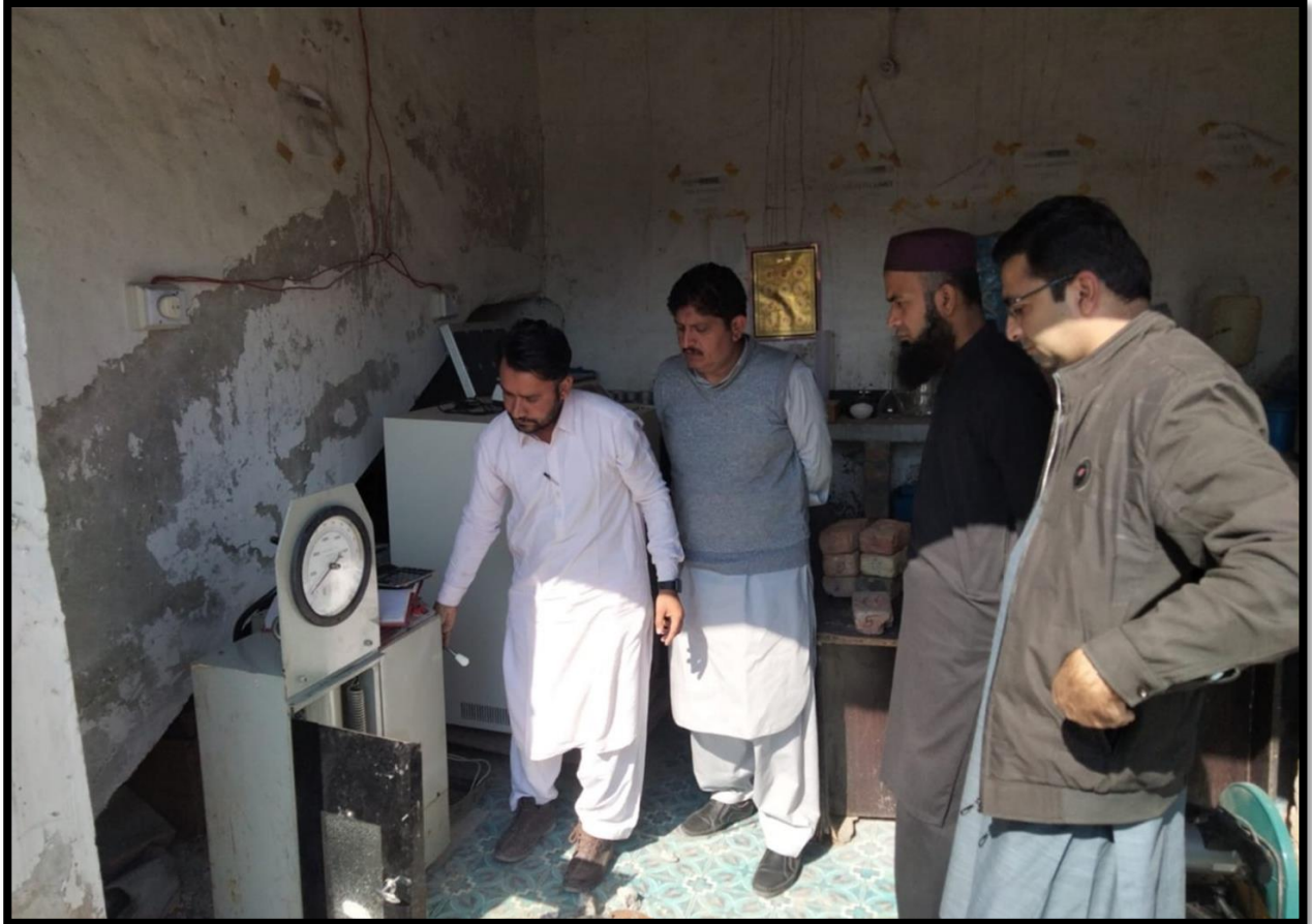
WW-09 (Zone-C) Cylinders testing of Compression for Sump of Disposal work in progress near Railway Station Jacobabad
