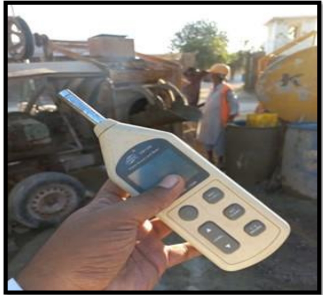
To check the Noise Pollution level with the help of (Digital Sound level).
