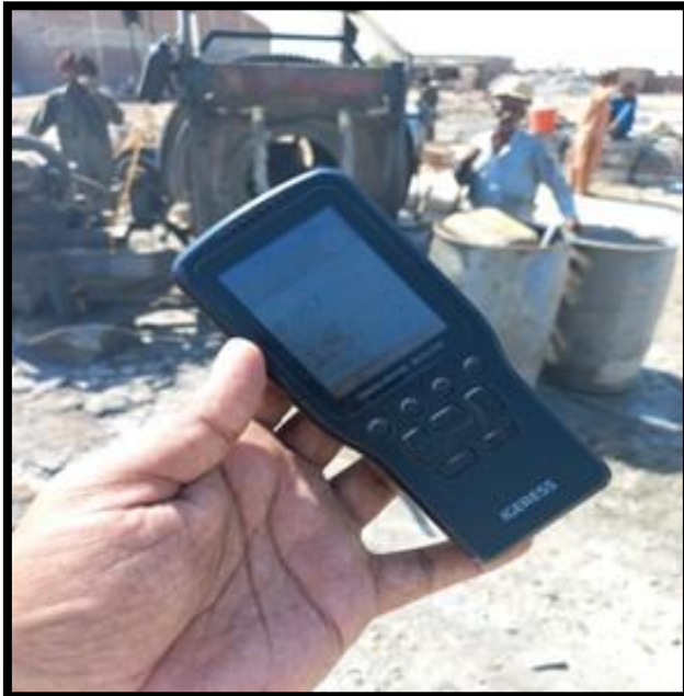
Monitoring of Air Pollution level during execution of work at Zone A Yard with the help of FORMALDEHYDE
