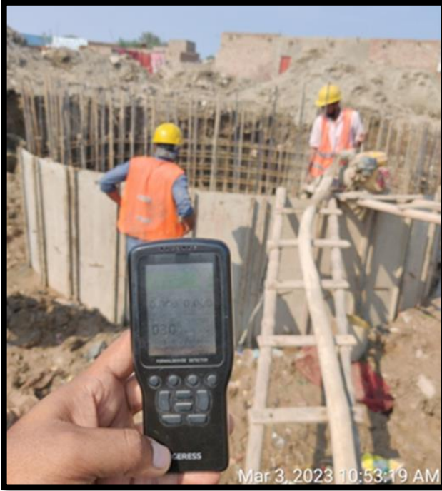
To check the Air Pollution level with the help of Formaldehyde Detector
