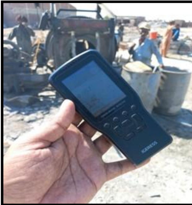
Monitoring of Air Pollution level during execution of work at Zone A Yard with the help of FORMALDEHYDE
