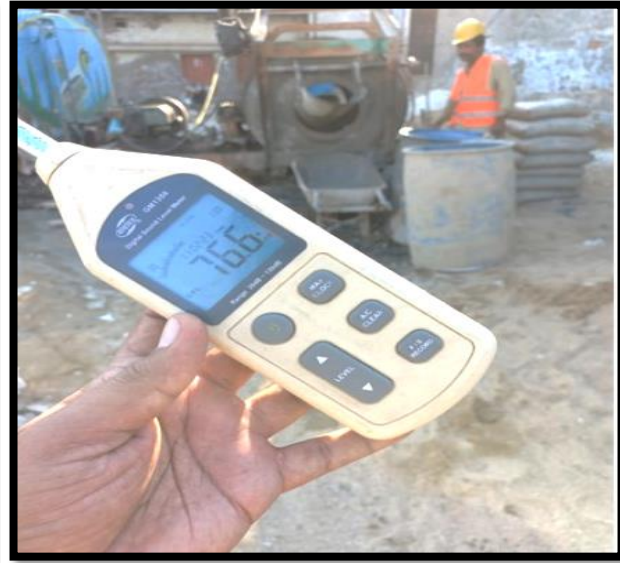
To check the Noise Pollution level with the help of (Digital Sound level Meter).
