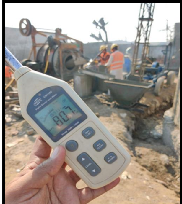
To check the Noise Pollution level with the help of (Digital Sound level Meter).
